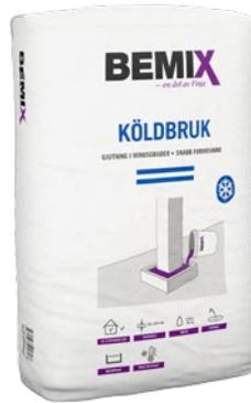
A ready-mixed, expanding cold-weather concrete for casting in sub-zero temperatures or when rapid formwork removal is required. Applications: underpouring for columns or prefab elements or when there is a requirement for rapid removal of formwork. Note! Cures in sub-zero temperature. For compressive strength see product data sheet at [bemix.se](http://bemix.se).
