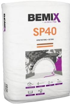
Sp40 shotcrete specially adapted for dry spraying. Used in repairs with requirements for minimal shrinkage and cracking such as e.g. lining of tunnels, reinforcement of columns, beams, quays and other concrete structures.
