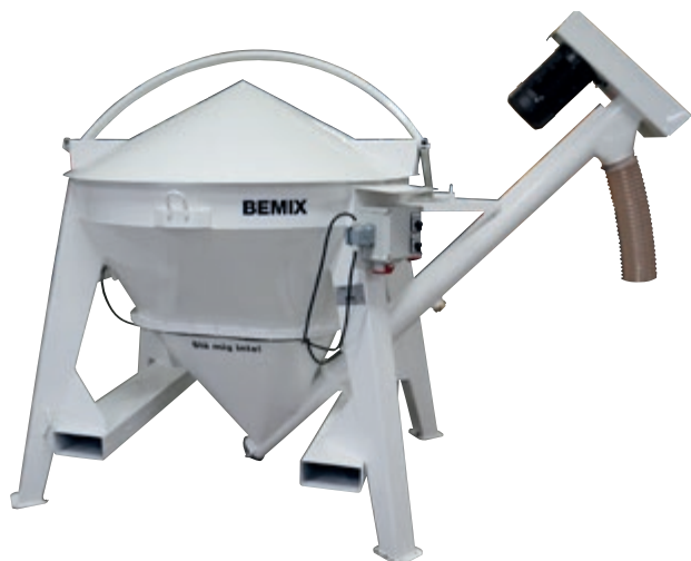
ST1 Big bag containers with screw pocket. Holds metric one ton.
